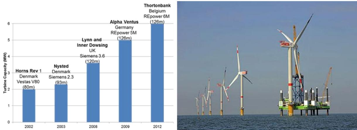
**Figure 4:** Europe’s more mature offshore wind industry is trending toward larger scale turbines that provide economies of scale. Turbine rotor diameter provided for each turbine. Germany (Alpha Ventus) and Belgium’s (Thorton Bank, installation pictured on right) first offshore wind farms successfully utilize larger-scale turbines (5MW or larger).
