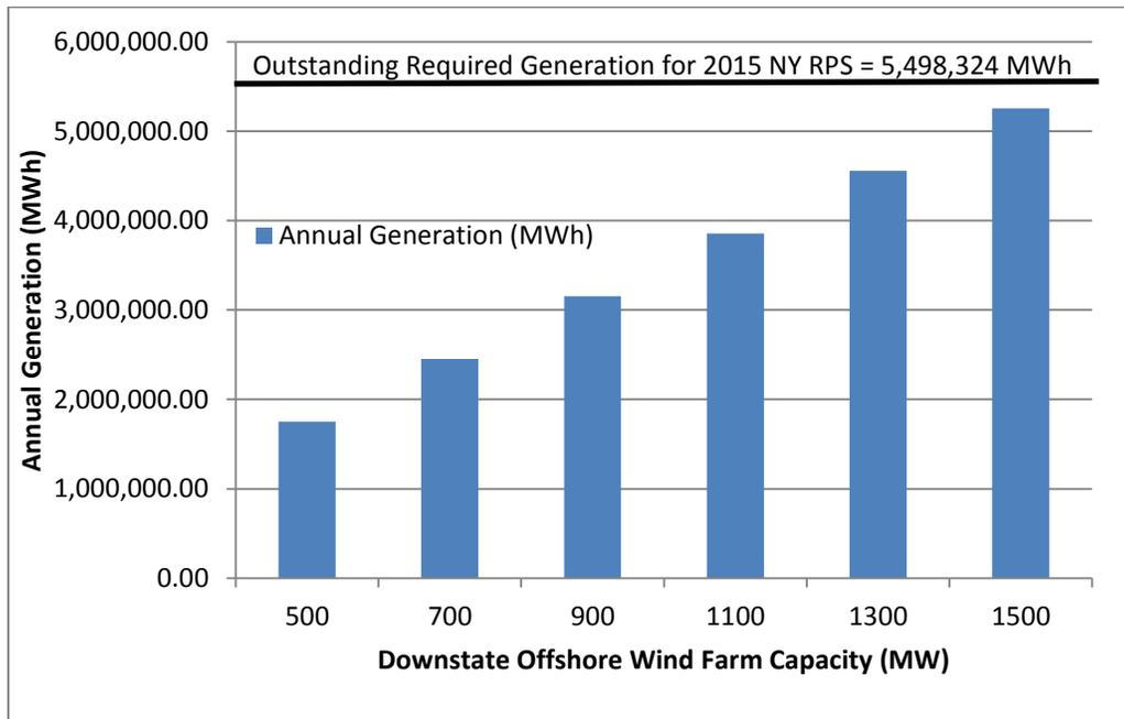
*Figure 7: Illustrative generation of an offshore wind farm (assumed capacity factor of 40%). Outstanding generation required for 2015 New York State RPS is included for reference.*
